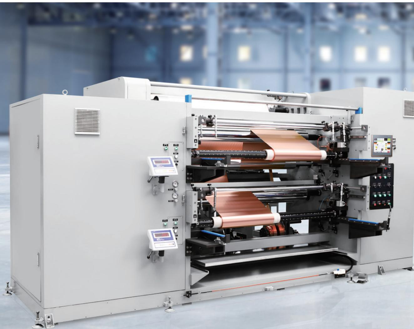
Full range of specifications and sizes were developed for high-tech industries. Our copper foil slitting machine are widely used in various types of fiberglass epoxy resin copper clad laminate, multilayer printed circuit board, flexible circuit board, IC-substrate, lithium-ion battery, and paper-phenolic resin copper clad laminate.
